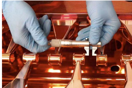
IH structure build by U. Ratzinger (GSI) Group for the BNL EBIS injector, 100 MHz
